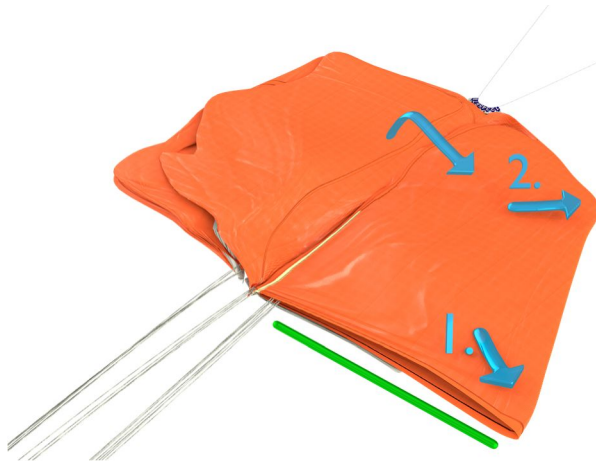
Picture 10 - Pulling out bottom and top corner.
