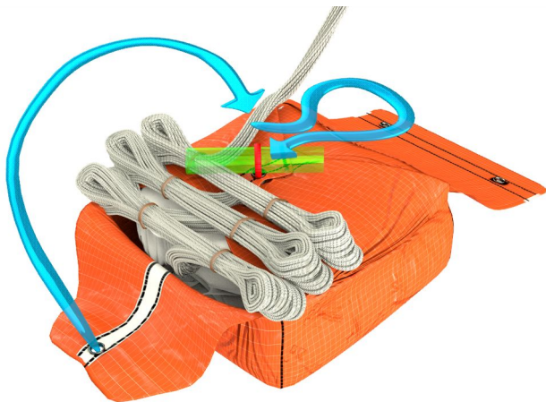
Picture 26 - Bundles inside, ready for final cover.
